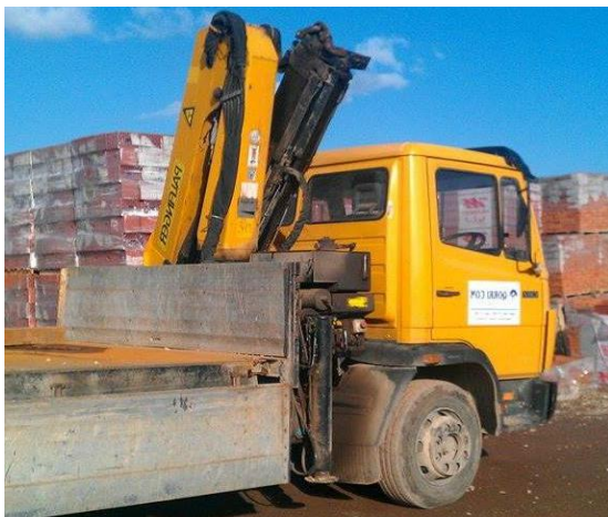
Fig.1. Crane mounted on the truck in the working environment
